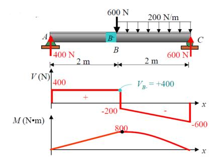
The maximum bending moment is 800 Nm located at the mid-length of the beam.
